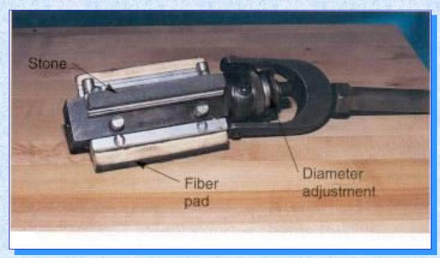
The adjustable stones lock into a preset position
