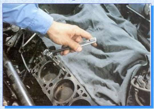
Run a tap through threaded holes to remove debris and locate damaged threads
